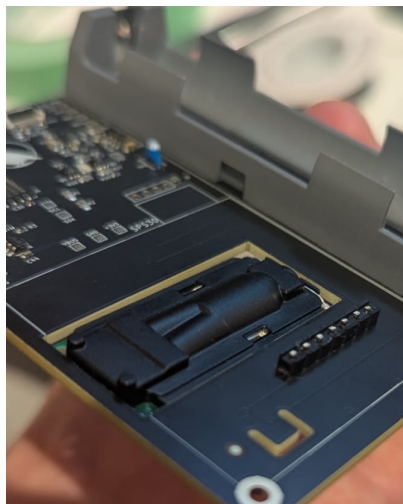
CO 2 sensor installed
